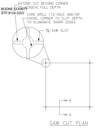
UNLESS SPECIFIED OTHERWISE, ALL LOOPS SHALL BE  $6^\prime \times 6^\prime$  SQUARE, CENTERED IN EACH LANE, WITH FOUR TURNS OF 14 AWG LOOP WIRE.
